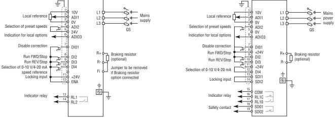
*Note*: For single-phase versions, the power supply is connected to terminals L and N.
