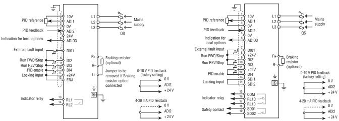
$\emph{Note}$ : For single-phase versions, the power supply is connected to terminals L and N.
