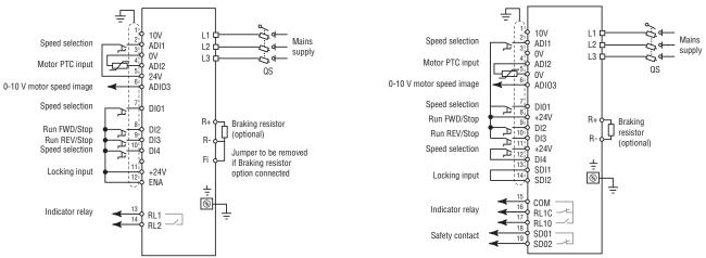
*Note*: For single-phase versions, the power supply is connected to terminals L and N.
