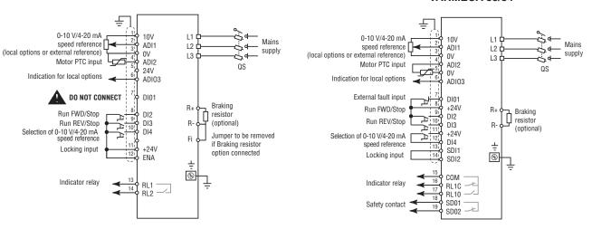
*Note*: For single-phase versions, the power supply is connected to terminals L and N.
