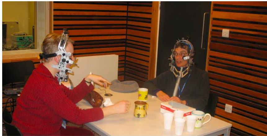
Figure 10. Two informants wearing a stabilizing headset for UTI during spontaneous discourse (from Scobbie et al. 2008).
