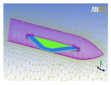
Figure6: Meshed model of Double delta wing body without domain.
