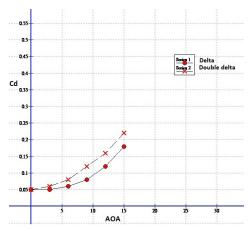
Comparison of drag curve for both the wing body configurations
