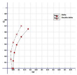
Comparison of drag polar for both the wing body configurations
