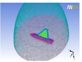
Figure6: Meshed model of double delta wing body with domain.
