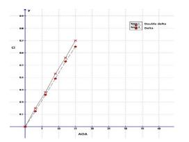
Comparison of lift curve of both the wing body configurations
