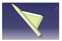
Figure1: Double delta wing body (lower surface).
