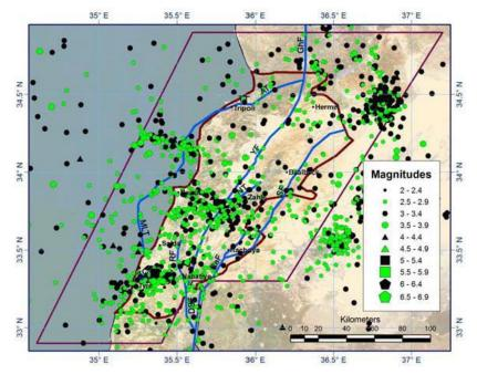
Figure 2-16 Instrumented Earthquake Events in and Around Lebanon between 1998 and 2009 with M ≥ 2 (Figure acquired from original source: Huijer et al., 2011)
