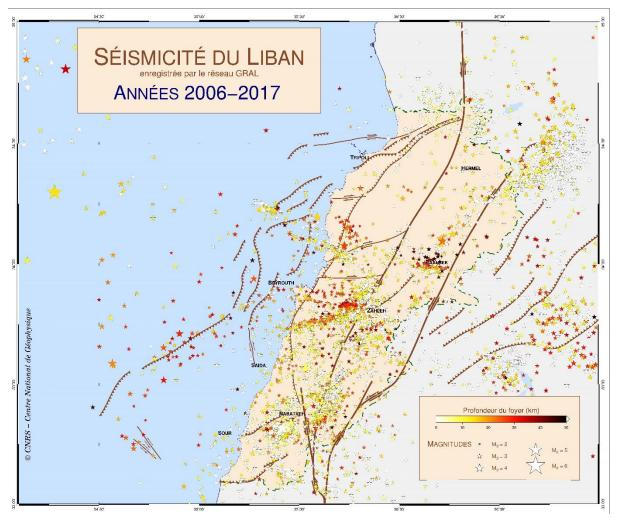
Figure 2-15 Main Structural Elements of Lebanon with Active Ones Shown in Red (CNRS, 2017)
