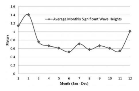
Figure 2-6 Average monthly significant wave heights offshore Beirut (Source: Aoun et al., 2013)
