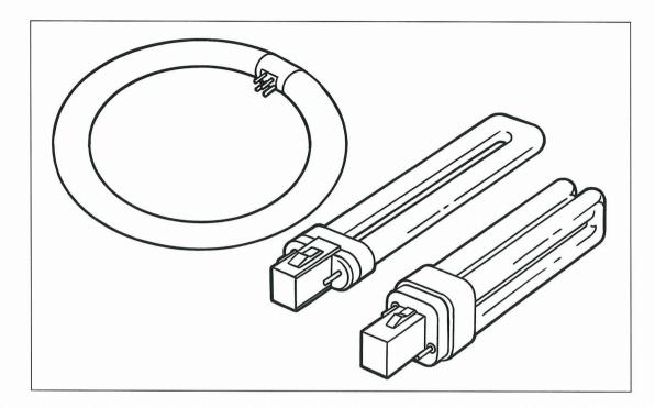
There are several types of compact fluorescent lamps. CFT or T4 twin-tube preheat lamps have starters in the base of the lamp and are available in 5, 7, 9, and 13 watts. CFQ or T4 or T5 quad-tube preheat lamps also have starters in the base and are most common in the 18- and 26-watt versions.
