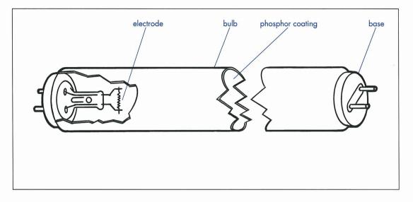
Fluorescent lamps are cylindrical glass tubes that are coated on the inside with phosphors. They contain a small amount of mercury and are filled with a small quantity of argon, a combination of argon and neon, or krypton gases. During operation, an electrical current passes through the lamp and the mercury is vaporized, producing ultraviolet light. The phosphor coating absorbs the ultraviolet light and re-radiates it as visible light.
