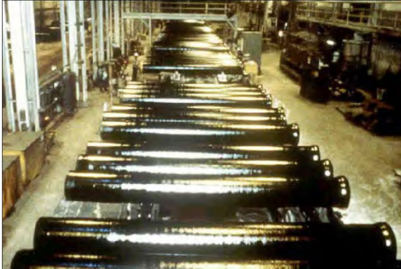
(Courtesy of Ductile Iron Pipe Research Association) Figure 3-10. Finished DIP at manufacturing facility.
