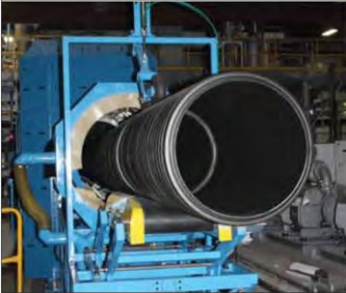
(Courtesy of Plastics Pipe Institute) Figure 3-15. Manufacture of a PW-HDPE.
