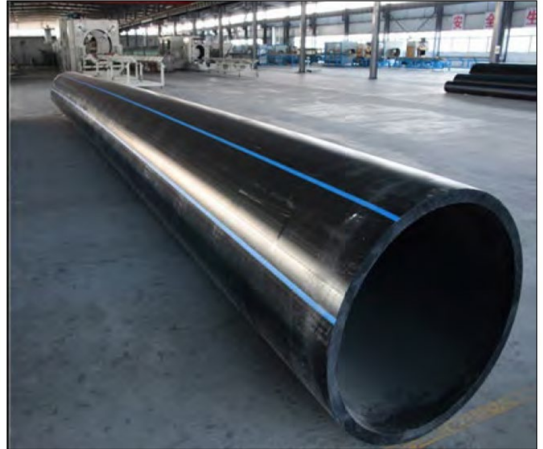
(Courtesy of Plastics Pipe Institute) Figure 3-12. Solid-wall HDPE at manufacturing facility.
