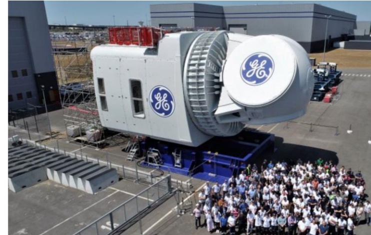
GE 12-MW Wind Turbine Nacelle – Haliade -X
