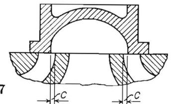
and fractions of an inch. It must be equal on both ends of the valve, because it is measured with the valve in its central position.
