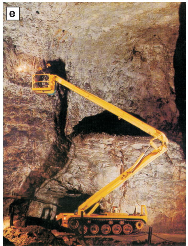
Figure 4 (continued): d) Scooptram close to one of the spodumene zone pillars illustrating the room and pillar method used at Tanco; e) Custom designed aerial lifts.
