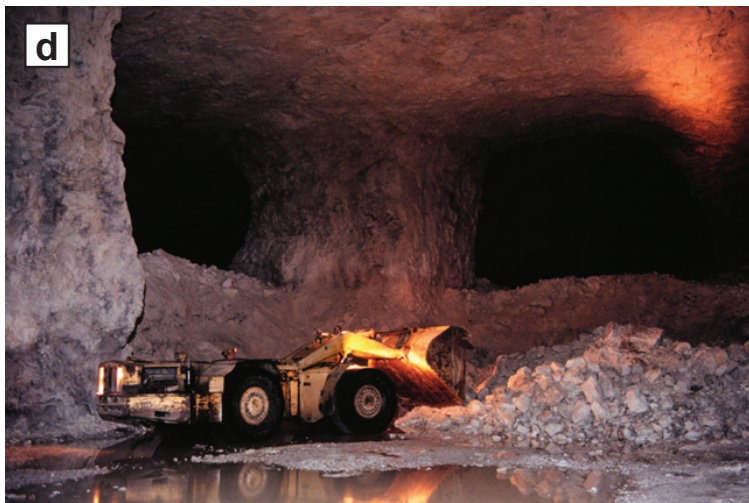
Figure 4 (continued): d) Scooptram close to one of the spodumene zone pillars illustrating the room and pillar method used at Tanco; e) Custom designed aerial lifts.
