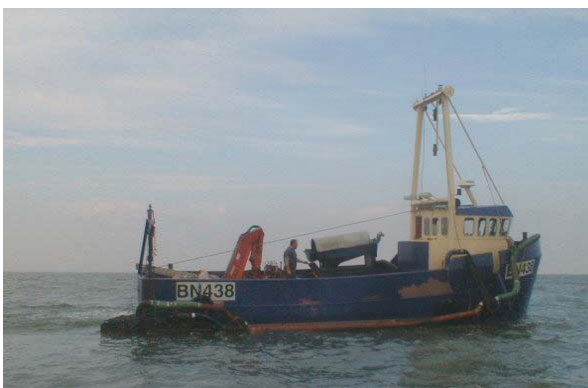
Plate 3. Cockle suction dredger. The suction pipe is ready for deployment to the seabed. The Wash. Image: Eastern Sea Fisheries Joint Committee.
