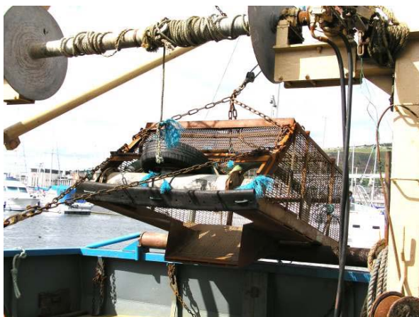
Plate 15. A hydraulic dredge used to capture razor clams ( Ensis spp) from Camarthen Bay, South Wales. 2003 Image: Blaise Bullimore/CCW
