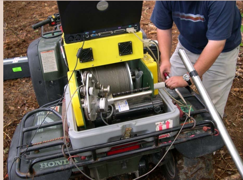
Winch, Data Processor and Laptop
