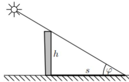
$$\begin{aligned}\tan \varphi &= \frac{h}{s} \\ \varphi &= \arctan \frac{h}{s} \\ \varphi &= \arctan \frac{40 \text{ m}}{67 \text{ m}} \\ \varphi &\approx 30,84^\circ\end{aligned}$$
