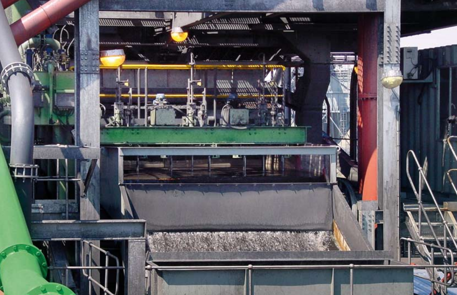
BATAAC Jig for coal separation, Leeuwplan, South Africa
