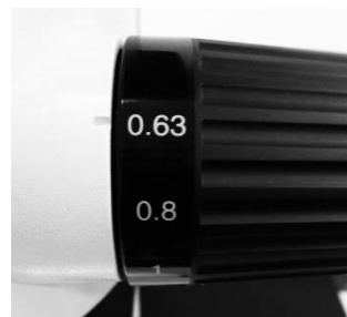
Figure 4-12: Setting the zoom factor at the MVX10.
