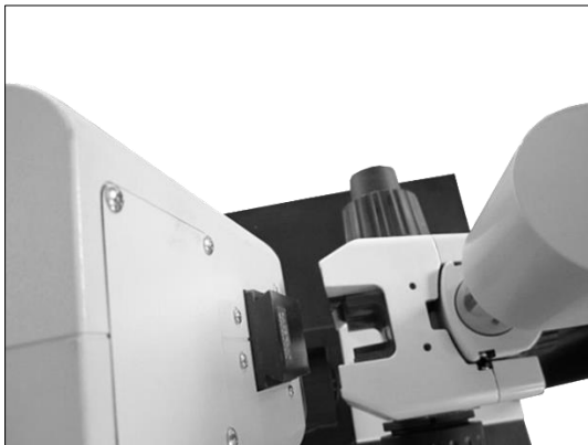
Figure 8-2: Release the MVX10 zoom body.
