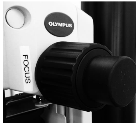
Figure 4-11: Knob at the focusing unit for lowering the lens into the imaging solution.
