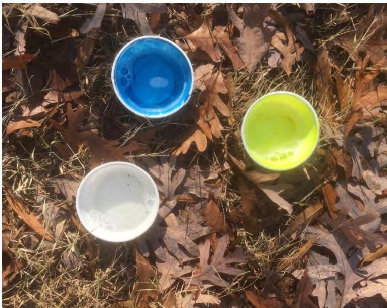
Figure 2. Bee bowls. 96.1-ml (3.25-oz) plastic “Solo® souflé portion cups” (original white, painted fluorescent blue, and painted fluorescent yellow).
