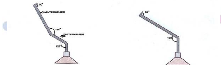
Figure 1: Diagrammatic representation of 2- and 3-bend cystitomes. In comparison to the 2-bend cystitome, the 3-bend cystitome has an extra bend at the centre. The three bends being at 90° at the bevel, 120° at the hub, and 150° at the centre point.
