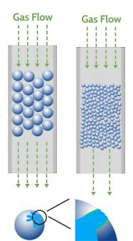
Breakthrough analysis is a powerful technique for determining the adsorption capacity of an adsorbent under flow conditions. Dynamic breakthrough adsorption provides many advantages over static adsorption measurements.
