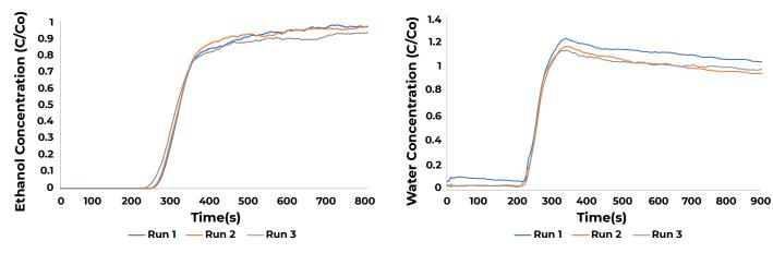
Figures: Ethanol (left) and water (right) multicomponent breakthrough curves collected at 50°C on zeolite 13X.
