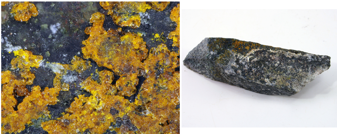
Figure 7: Detail image of huemulite (SEM-EDS/Raman conf.), field of view approx 2.4 mm (left). Macro photograph of the complete sample with metamunirite (Raman conf.), sample width \approx 3.5 cm.
