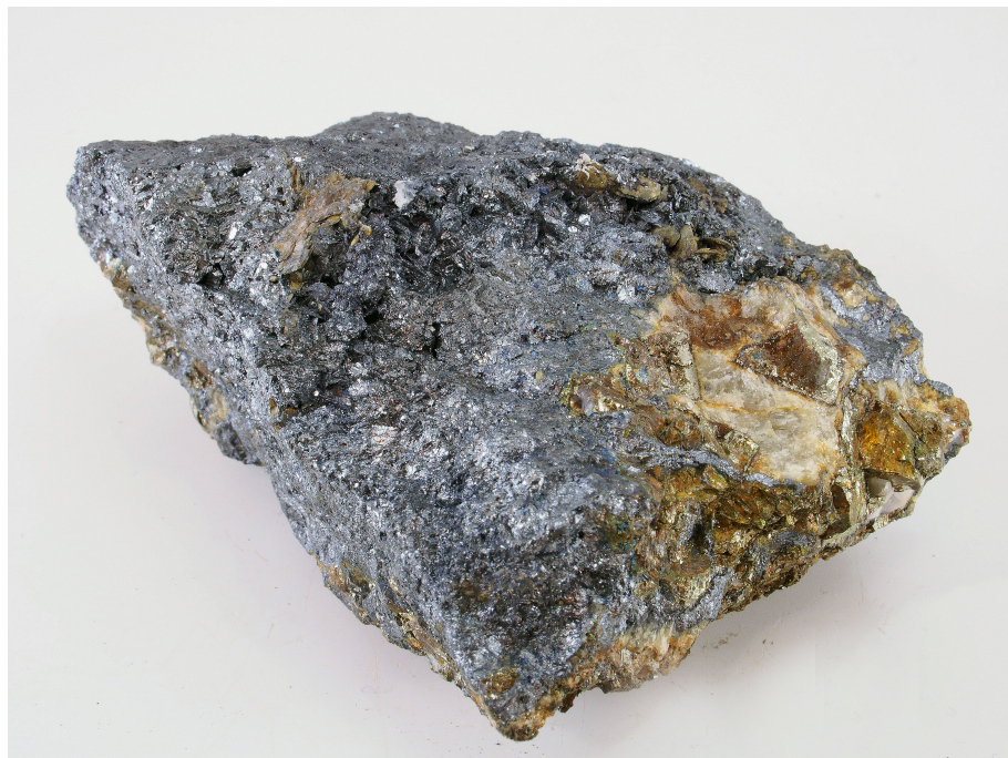
Figure 17: Hand sized sample with massive semseyite and semseyite in crystals embedded in a pyrite vein of siderite matrix.
