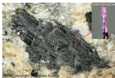
Fig1. (a) The aggregates of dumortierite crystals occurring in pegmatite from Krucze Rocks, Karpacz - Wilcza Poręba. (b) Single crystal of dumortierite for which the crystal structure analysis was described in this work.
