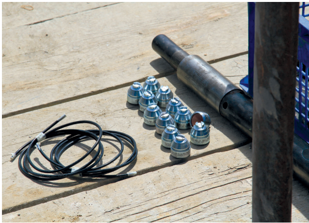
Fig. 1-2: 12 “shaped charge” explosives with the shot tube for borehole perforation on the right hand side and the fuses on the left hand side, just before assembly.
