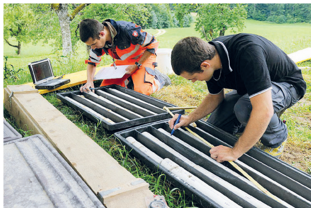
Fig. 3-1: Standard core mapping at the drilling site near Derrière-Monteri. (Photo © Comet Photoshopping GmbH)
