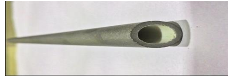
Fig. S4. In-house synthesized composite V-Fe membrane.
