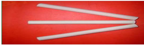
Fig. S3. In-house synthesized composite alumina tubes.
