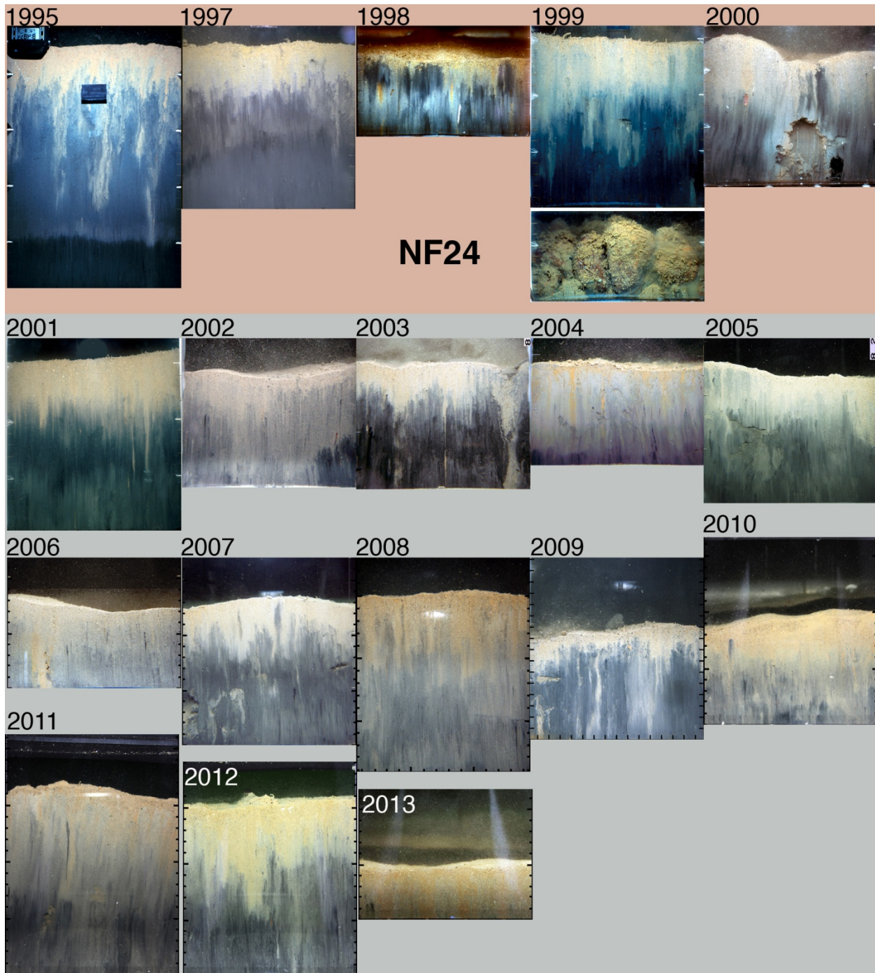
Figure 3-23. Mosaic of SPI from station NF24 for all years. Baseline years are up to 2000. Post-baseline years are from 2001. Sediment grain-size at NF24, within a half km of the outfall, is finest of all nearfield stations. Surface sediments are consistently light in color indicating there has been no accumulation of organic matter post-baseline. Scale along the side of each image is in cm.
