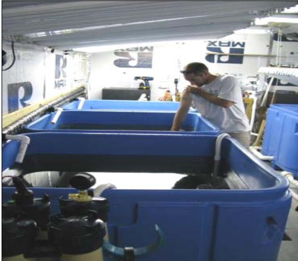
Fig. 9.3. SCCF Marine Lab mesocosm facility, three-300 gallon insulated holding tanks refitted with new circulating pumps/filters for holding urchins and macroalgae.
