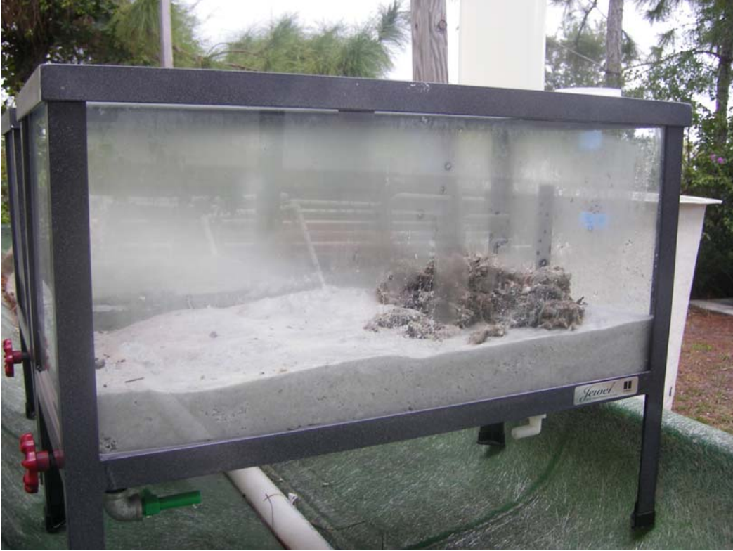
Figure 6.3 – Laboratory decomposition experiment using microcosms. Prewighed samples of algae were placed in the aquaria and flushed with seawater. Nutrient concentrations were determined from the effluent.
