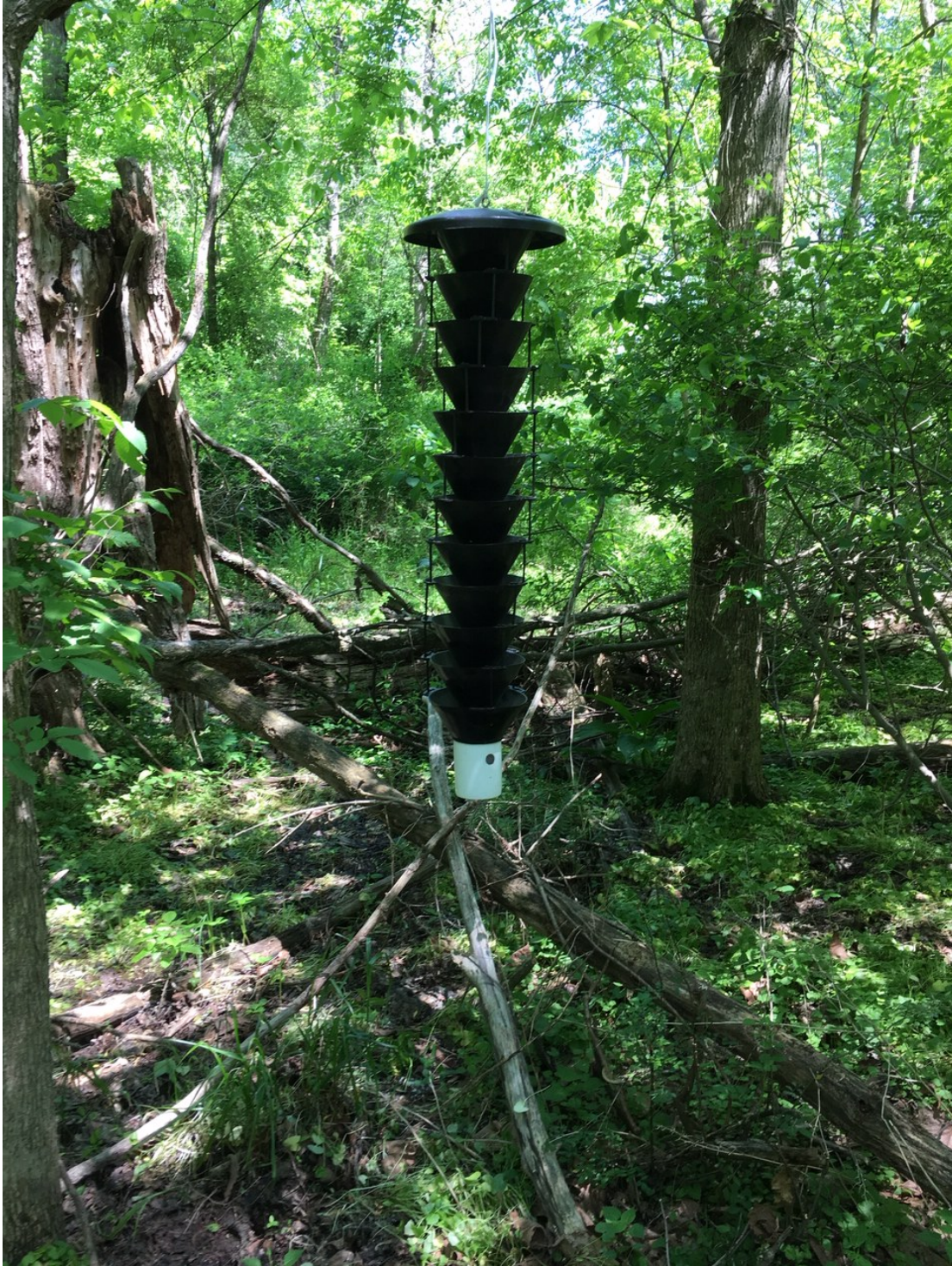
Figure 3-10. Lindgren Funnel set at the Raystown Branch of the Juniata River at the Nature Trail area in the Raystown Lake Project Area, PA.
