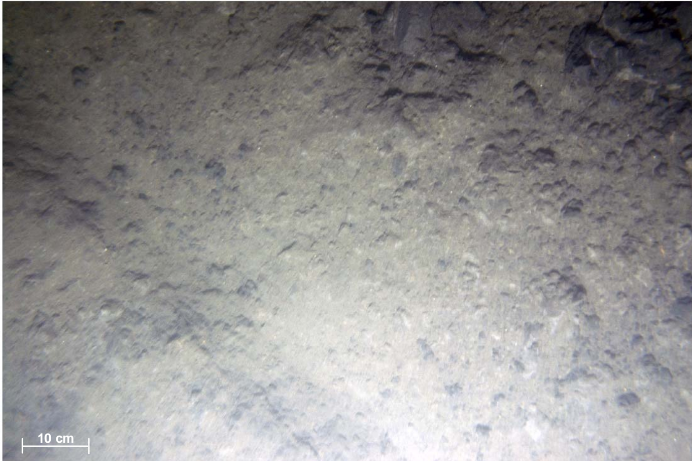
Figure 3-27. This plan view image from Station BE-04 shows the sediment surface littered with consolidated clay clumps from the recent disposal operations.
