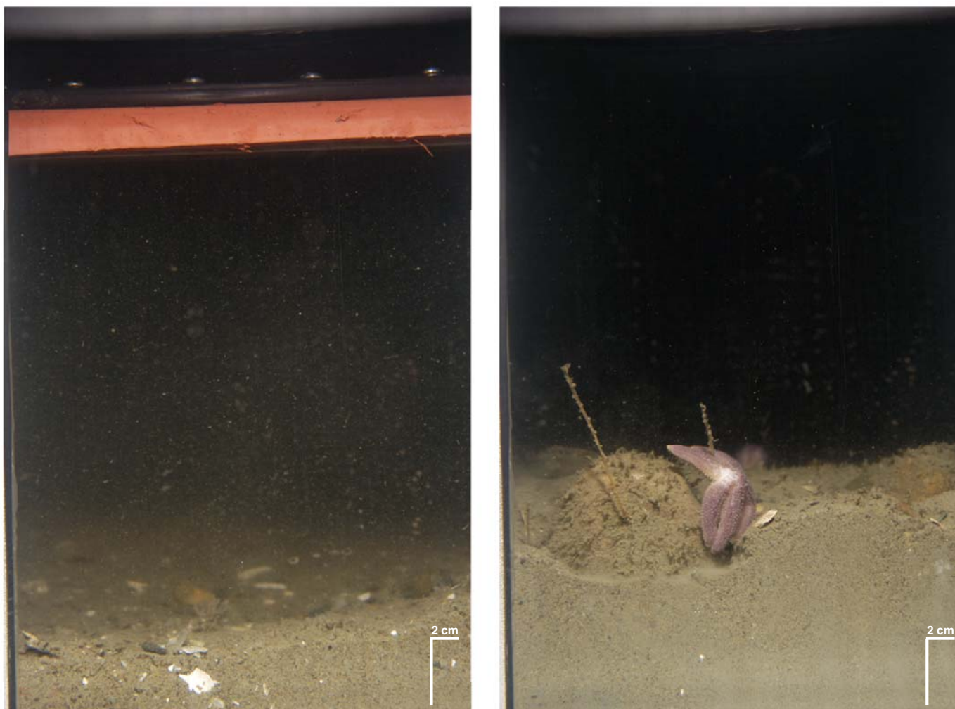
Figure 3-3. SPI images from Station REF-NE-03 (left) and Station REF-NE-04 (right) show shell hash and small rocks on the surface of the sandy bottom, which limited camera prism penetration.
