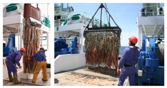
Figure 3. Rock dredge (left) and scallop dredge (right)
