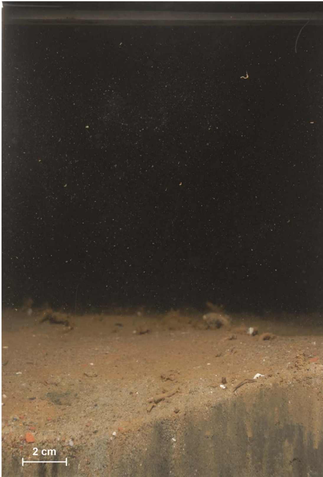
Figure 3-18. Profile image from PRA 1 Station 2010-03 showing dark (reduced), sandy dredged material with a relatively shallow aRPD depth of 0.6 cm
