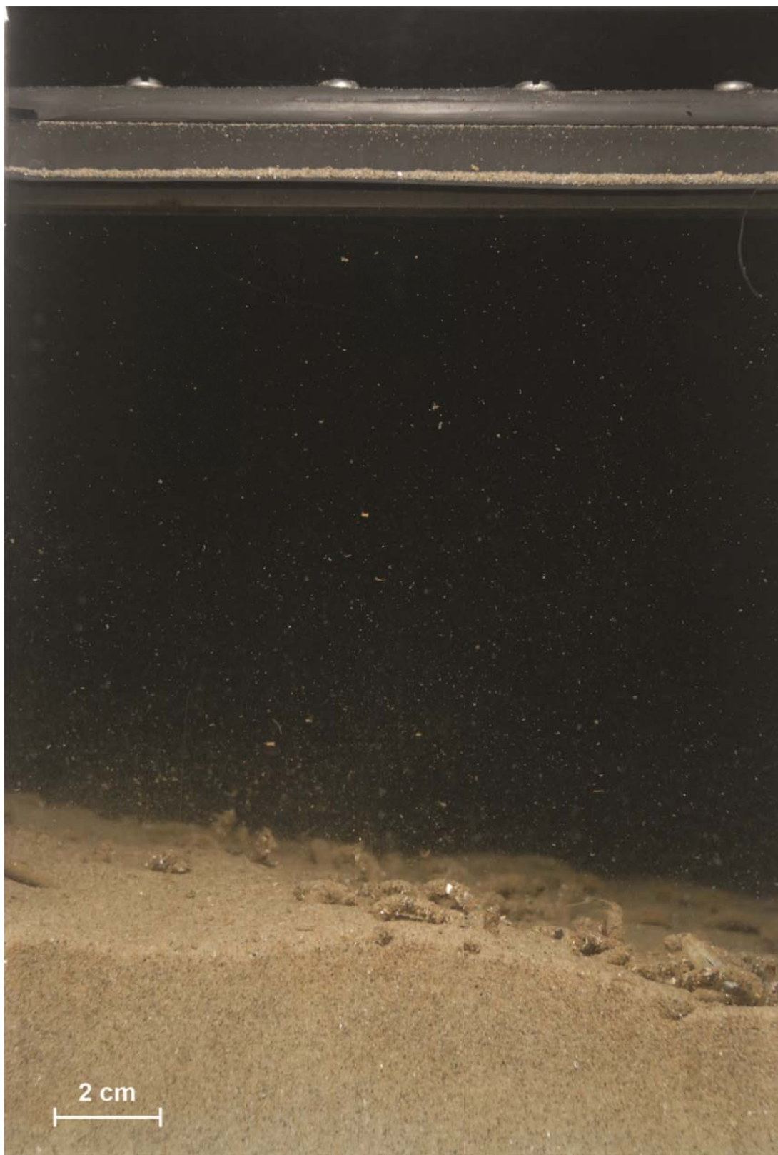
Figure 3-2. Profile image from PRA 1 Station 2010-07 illustrating fine sand (3 to 2 phi) that is relatively free of fine grained sediment (referred to as “clean” fine sand)
