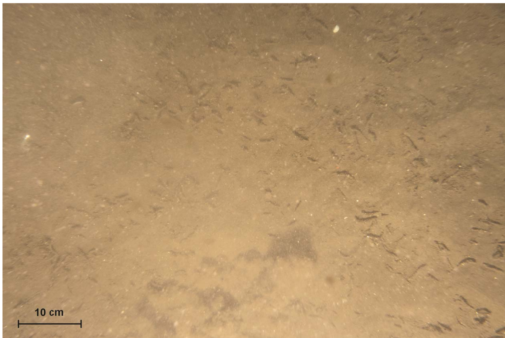
Figure 3-10. Plan-view image providing an example of muddy fine sand at PRA 1 Station 2010-02. Large worm tubes are also visible on the sediment surface.
