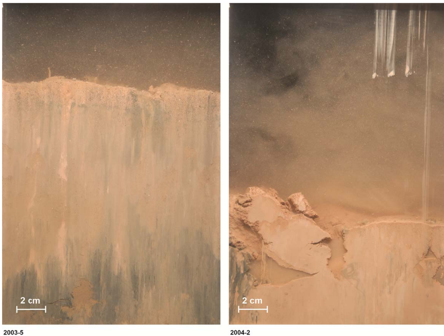
Figure 3-32. Profile images from Stations 2003-5 (left) and 2004-2 (right) showing red clay having a grain size major mode of >4 phi
