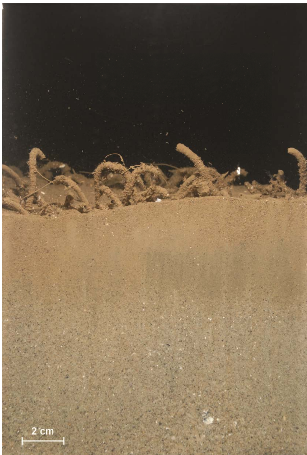
Figure 3-4. Profile image illustrating muddy fine sand at Station 2010-02 within PRA 1. A surface layer of brown silt/clay, with numerous large worm tubes, overlies fine sand at depth.
