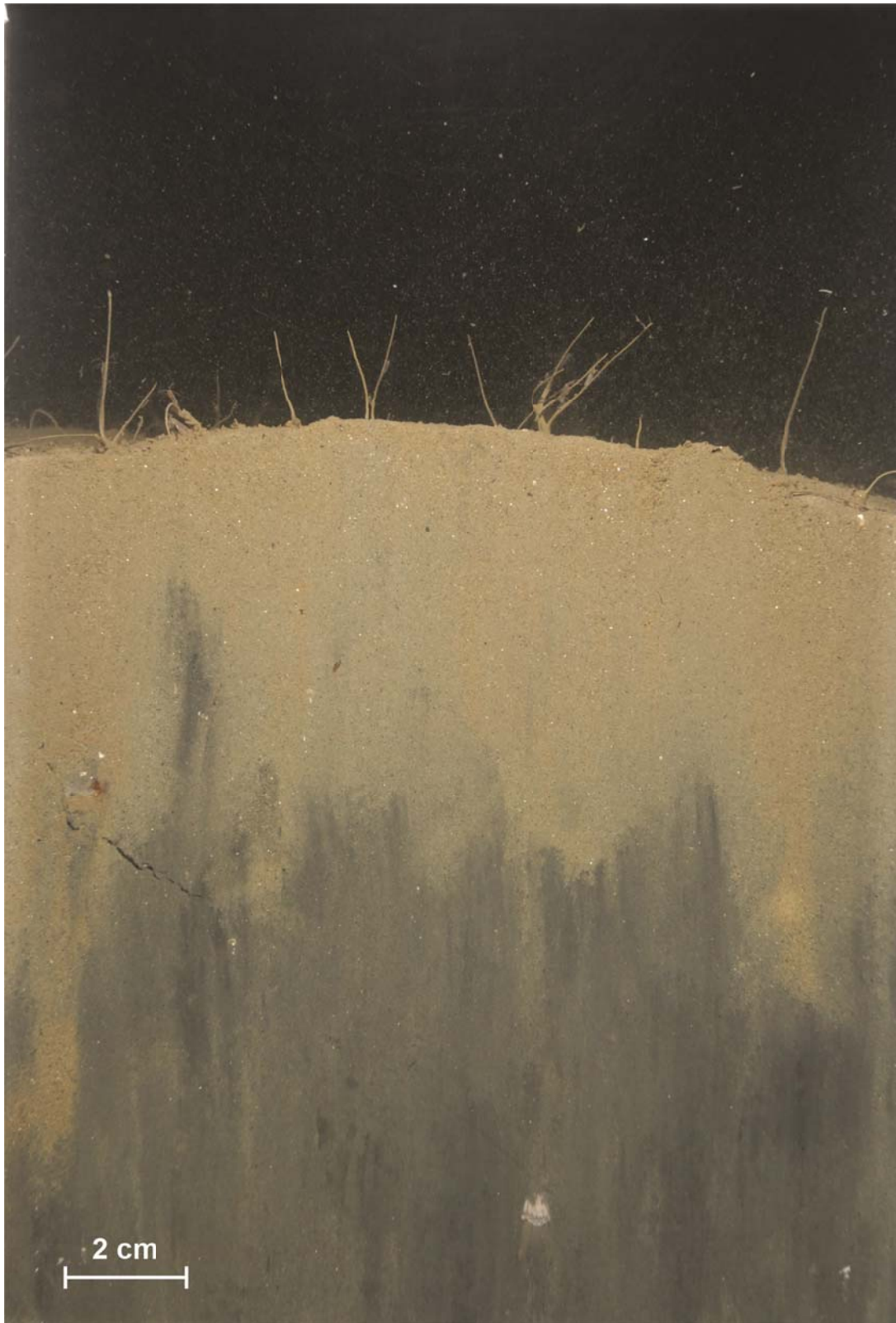
Figure 3-31. Profile image illustrating sand-over-mud layering at Station 03. Similar layering characterized nearby Station 02.
