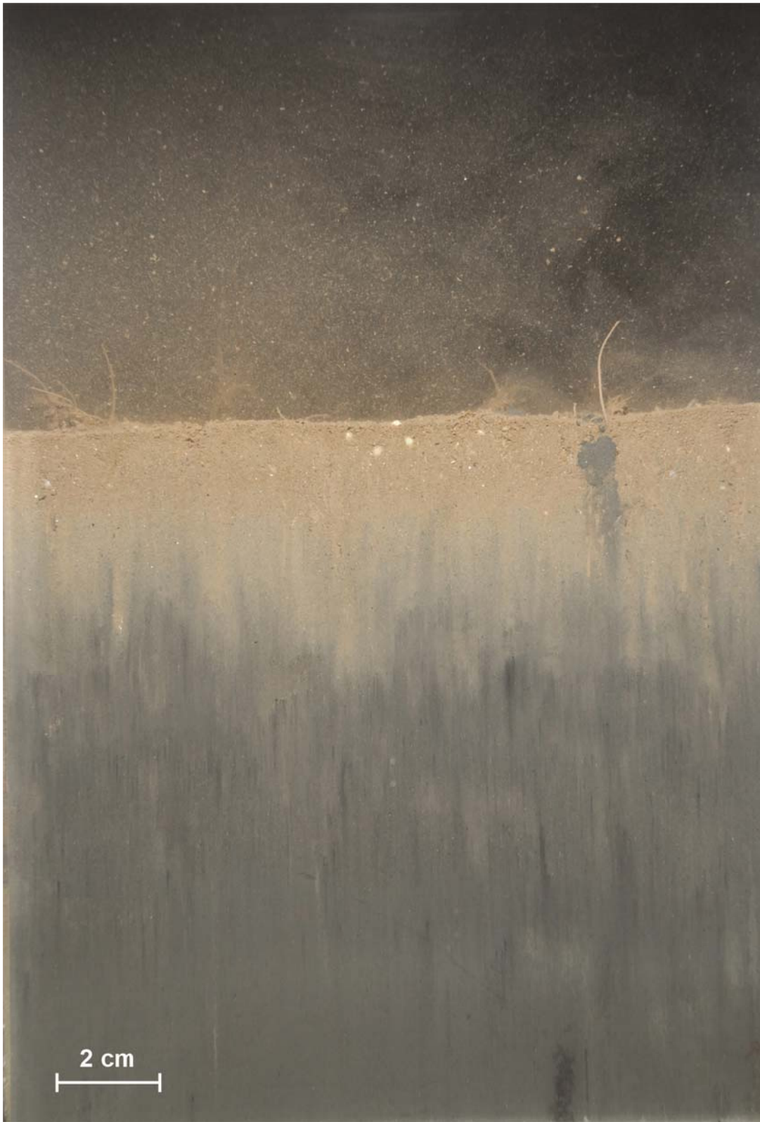
Figure 3-33. Soft, muddy, relict dredged material at Station 18 located near the center of PRA 6
