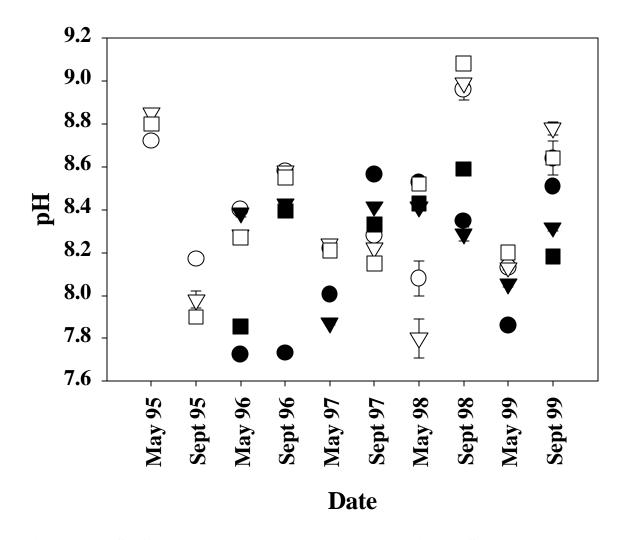
**Figure 2-51.** Surfzone and Nearshore Bottom Water pH (Mean<u>+</u>SE). Filled symbols = Surfzone, Open symbols = Nearshore Bottom water; Circle = South Area, Inverted Triangle = Middle Area, Square = North Area.
