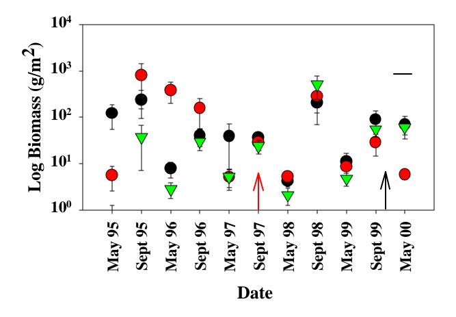
Figure 2-10. Nearshore Biomass (Grams/m<sup>2</sup>+SE) by Date. Black Circles = South Area, Red Circles = Middle Area, Green Triangles = North Area; Red arrow indicates South Area nourished; Black arrow indicates Middle Area nourished; Bar indicates a significant (p<0.0125) linear contrast between means.
