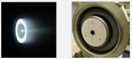
Advanced Thrusters and Successful testing a new 12.5k Hall Thruster
