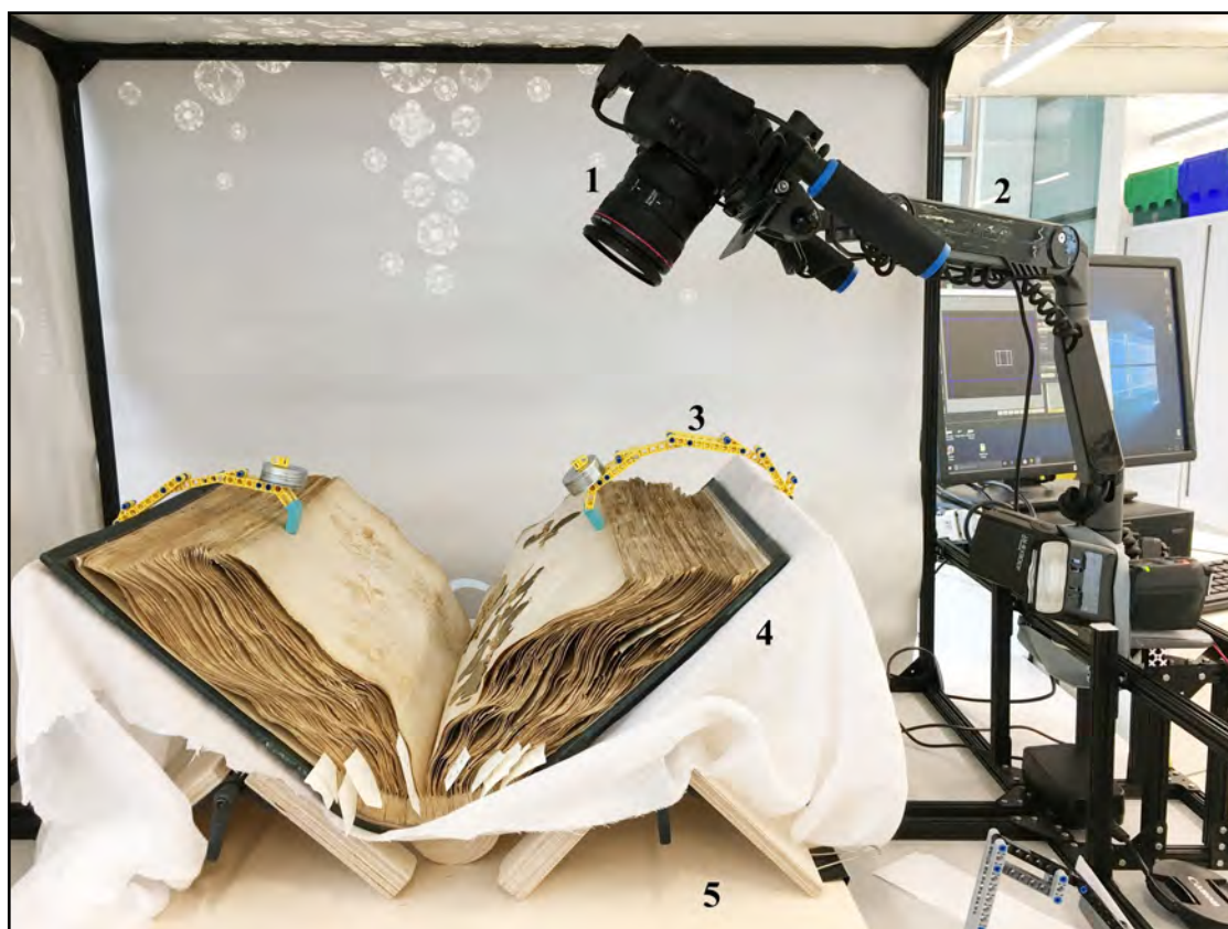
Figure 1. The Herbarium Imaging Equipment (HerbIE) including DSLR camera (1), adjustable swivel arm (2), Flecs (3), Book cradle (4), and turntable (5).
