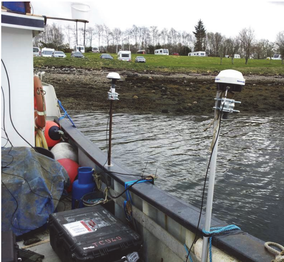
Figure 5.1. Configuration of Hemisphere VS300 Vector Sensor antennas, with transducer mounted outboard between the two and steering DGPS receiver above the main antenna (in bucket).
