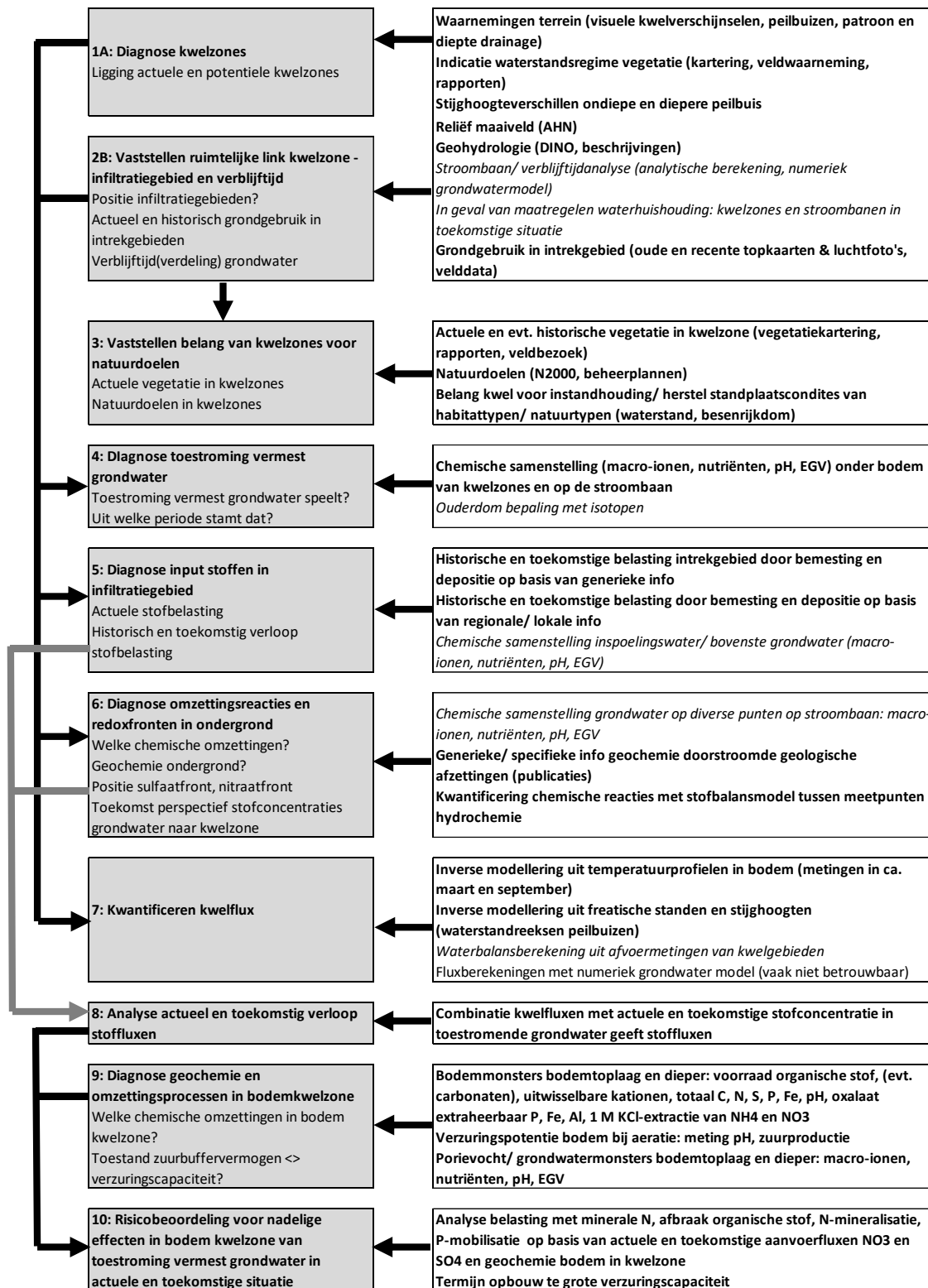
Figure 3-1: Flow chart for assessment of the effects of eutrophied groundwater in seepage zones of brook valleys. Bold = relatively easy to implement; italics = requires large effort/ relatively expensive.
