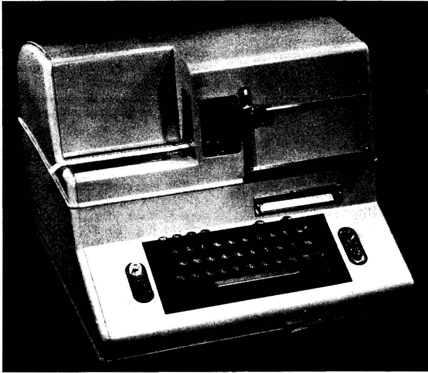
Figure 10-34.— Send/receive typing reperforator TT-253/UG. 50.116
