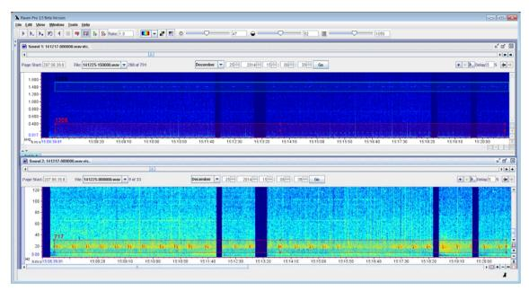
Figure 4: Example of time aligned spectra displayed in the software Raven Pro. The upper spectrogram is the 10-kHz down-sampled data and was used to identify mid-frequency vocalizations from minke whales (blue box) and humpback whales (red box). The lower spectrogram is the 1-kHz data and was used to identify calls from fin whales (red box) and blue whales, and also provided context when identifying the mid-frequency calls.
