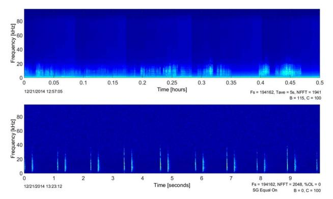
Figure 12: Sperm whale echolocation clicks recorded with SG203 on 21 December 2014. The first of two closely spaced clicks is the actual click; the following, longer duration signal is likely a bottom reflection.
