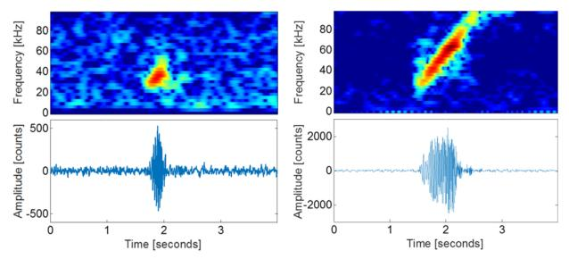
Figure 9: Blainville's beaked whale echolocation click (left) and CSBW echolocation click (right) recorded withSG203. Both examples are high-pass filtered at 10 kHz. Amplitude range of waveform is  $\pm$ 32,768 digital counts (16 bits).
