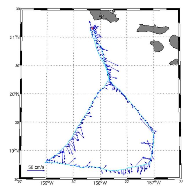
Figure 8: Depth-averaged currents measured with SG203.
