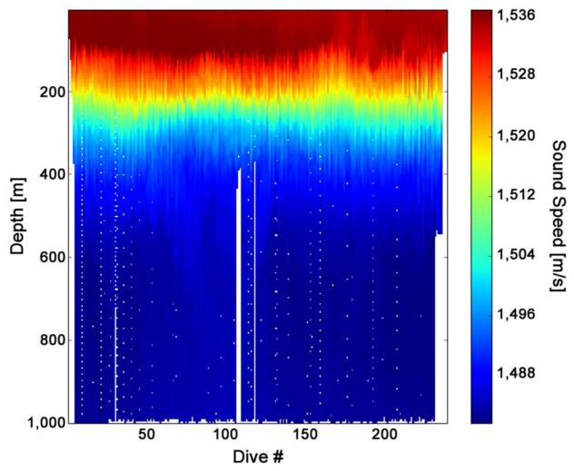
Figure 7: Sound-speed profiles recorded with SG203.
