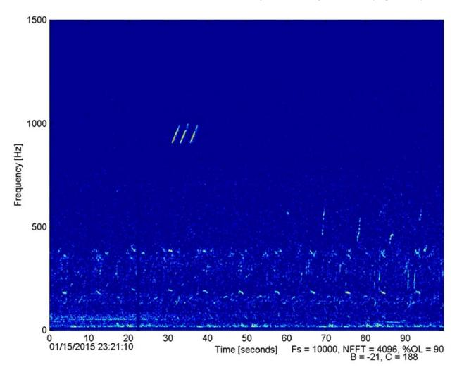
Figure 35: Active U.S. Navy sonobuoy sounds recorded with SG203 on 15 January 2015. The lowfrequency NWPBW calls with harmonics and humpback whale song is also visible in the lower half of the spectrogram.
