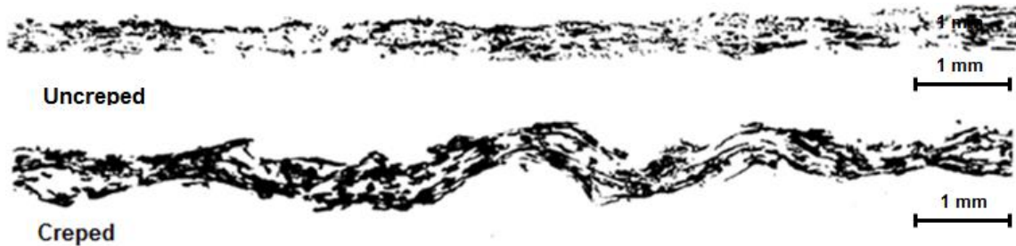
Fig. 15. The cross-sectional images of uncreped and creped paper (Welsh 1965)
