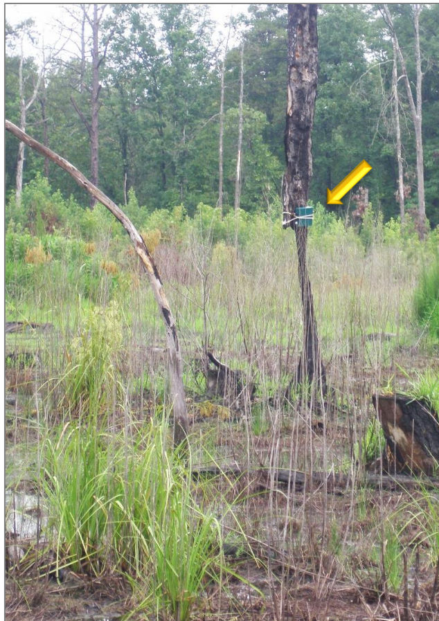
Figure 17. Photograph of froglogger positioned on a dead tree in an enhancement wetland (Block T).
