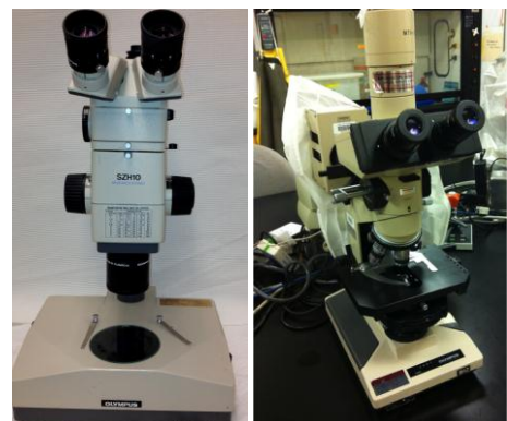
Figure 9. Dissecting (left) and compound (right) microscope.
