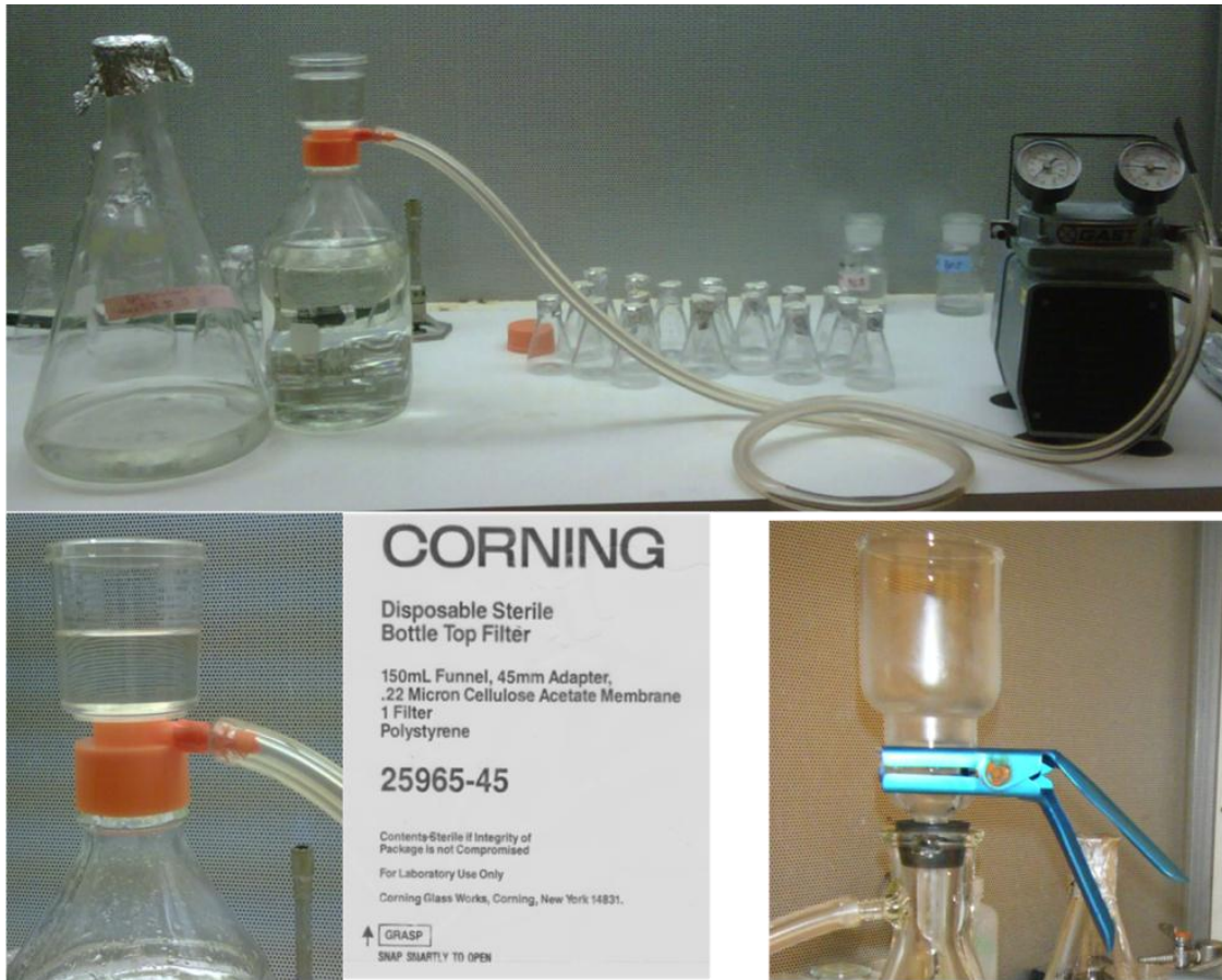
Figure 4. Vacuum pump assembly for filter sterilization (0.2 \mu\text{m} ) of nutrient media (top). Filter assemblies can be disposable (left, bottom) or reusable (right, bottom).
