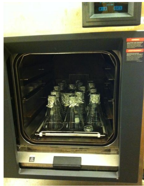
Figure 3. Autoclave for sterilization of seawater and glassware.
