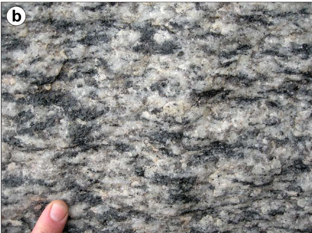
Figure 27. a – Sampling location 23091008 with Reinoksfjellet in the background. b – Coarse-grained biotite granite gneiss at sampling location 23091008.
