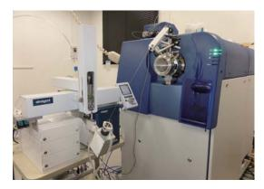
Figure 2. Triple TOF LC/MS/MS System
