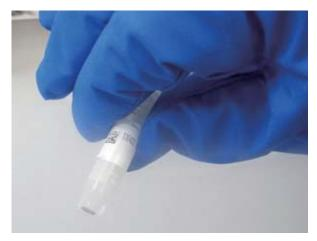
Figure 3. Cryotube with 2D barcode. Each sample is printed with a unique barcode and is managed using a database.
