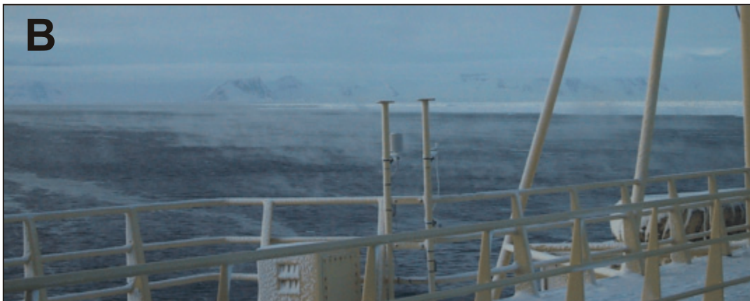
Figure 7. A) The NBP “science” mast, with port and starboard anemometers and shortwave, longwave, and PAR sensors mounted to the railing. B) The temperature, relative humidity, and longwave radiation sensors, with sea smoke in the background.
