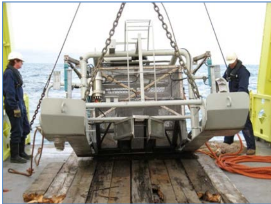
Figure 13. Megabenthos: Deep Digging Dredge (Triple-D: 2008 version: ~ 1500 kg).
