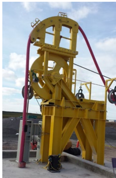
Sheave Stand Assembly
