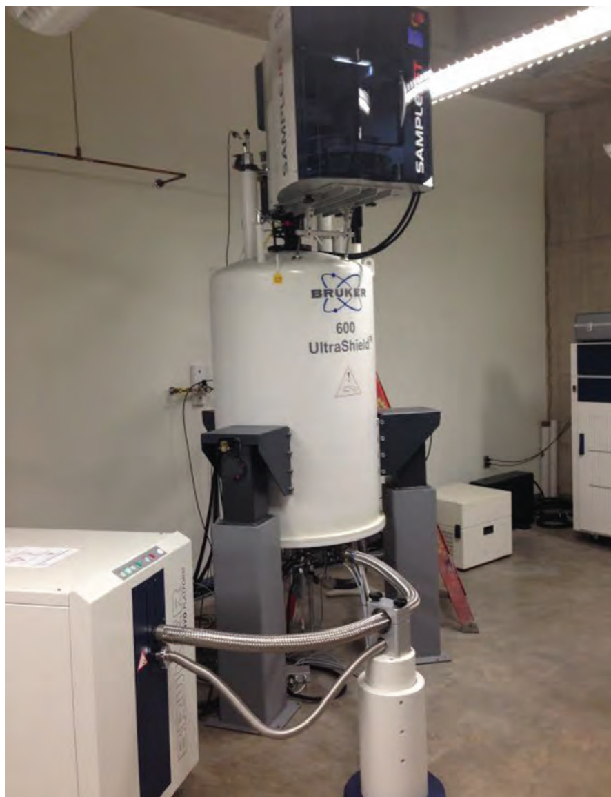
Nuclear magnetic resonance spectroscopy machine used to detect biological molecules (metabolites) in blood samples that may hold promise as a technique to assess the nutritional and health status of animals. Photo by Bob Garrott, Montana State University.
