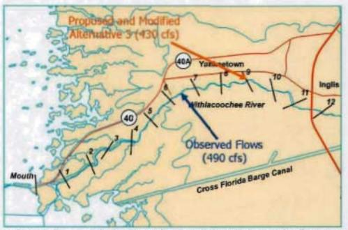
Figure 5-20. Median monthly locations of surface 0.5 ppt isohalines for flow scenarios, October 2000, during low flow conditions. Proposed and Modified Alternative 3 scenarios include conditions which will not be implemented (the 400 cfs one day/week discharge to the Barge Canal), so that the location of the isohaline resulting from the observed flows should be considered.
