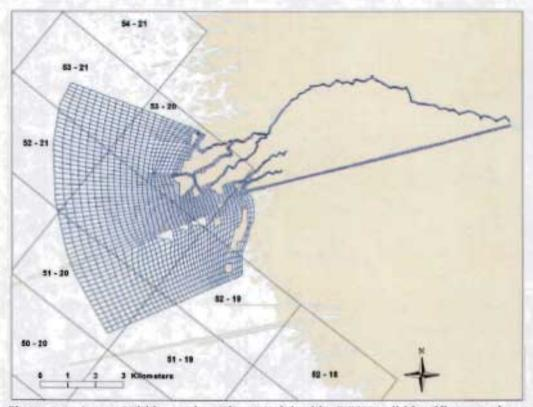
Figure 4-5. Lower Withlacoochee River Model grid. GCSM cell identifiers are shown in black.
