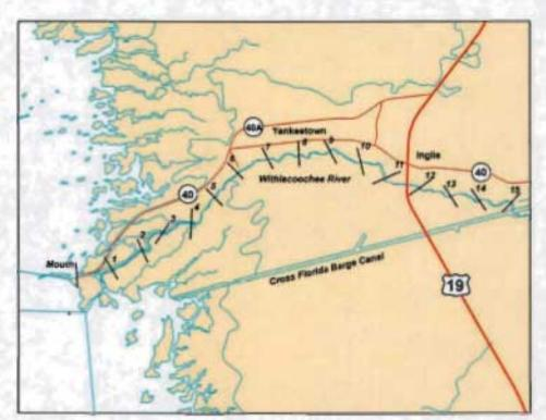
Figure 5-1. River kilometer system for the Lower Withlacoochee River.
