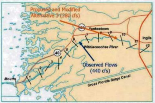
Figure 5-22. Median monthly locations of surface 0.5 ppt isohalines for flow scenarios, December 2000, during low flow conditions. Proposed and Modified Alternative 3 scenarios include conditions which will not be implemented (the 400 cfs one day/week discharge to the Barge Canal), so that the location of the isohaline resulting from the observed flows should be considered.
