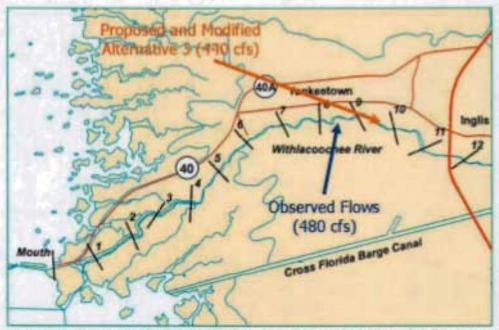
Figure 5-21. Median monthly locations of surface 0.5 ppt isohalines for flow scenarios, November 2000, during low flow conditions. Proposed and Modified Alternative 3 scenarios include conditions which will not be implemented (the 400 cfs one day/week discharge to the Barge Canal), so that the location of the isohaline resulting from the observed flows should be considered.
