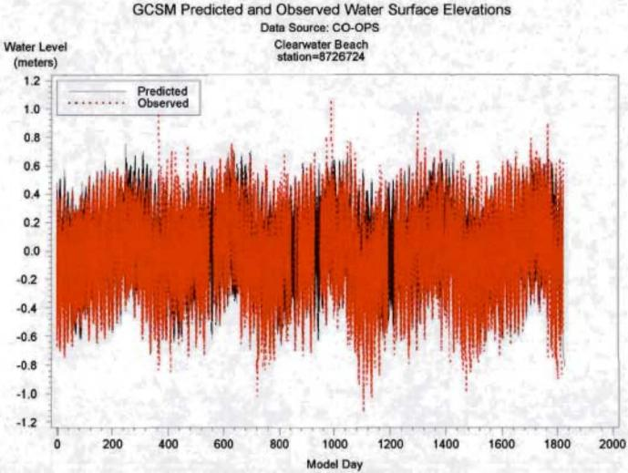
Figure A-3. Time series of predicted and observed tidal record at Clearwater Beach.
