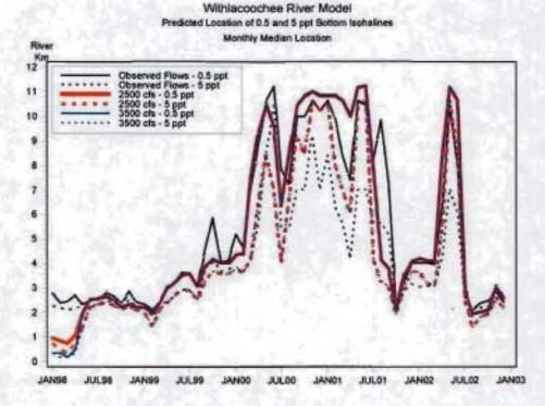
Figure 5-24. Monthly median locations of bottom 0.5 and 5 ppt isohalines, baseline, 2500 cfs alternative, and 3500 cfs alternative.
