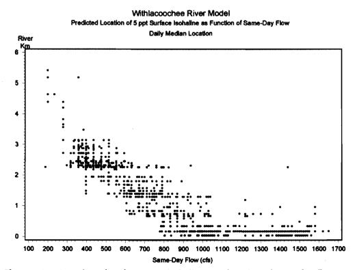
Figure 5-37. Location of surface 5 ppt isohaline as a function of same-day flow.
