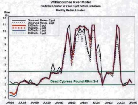
Figure 5-35. Monthly median locations of bottom 2 and 3 ppt isohalines, baseline, 2500 cfs alternative, and 3500 cfs alternative.
