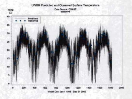
LWRM Predicted and Observed Surface Temperature Data Severe: COAST station=8
