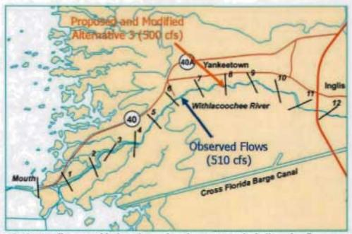
Figure 5-19. Median monthly locations of surface 0.5 ppt isohalines for flow scenarios, September 2000, during low flow conditions. Proposed and Modified Alternative 3 scenarios include conditions which will not be implemented (the 400 cfs one day/week discharge to the Barge Canal), so that the location of the isohaline resulting from the observed flows should be considered.
