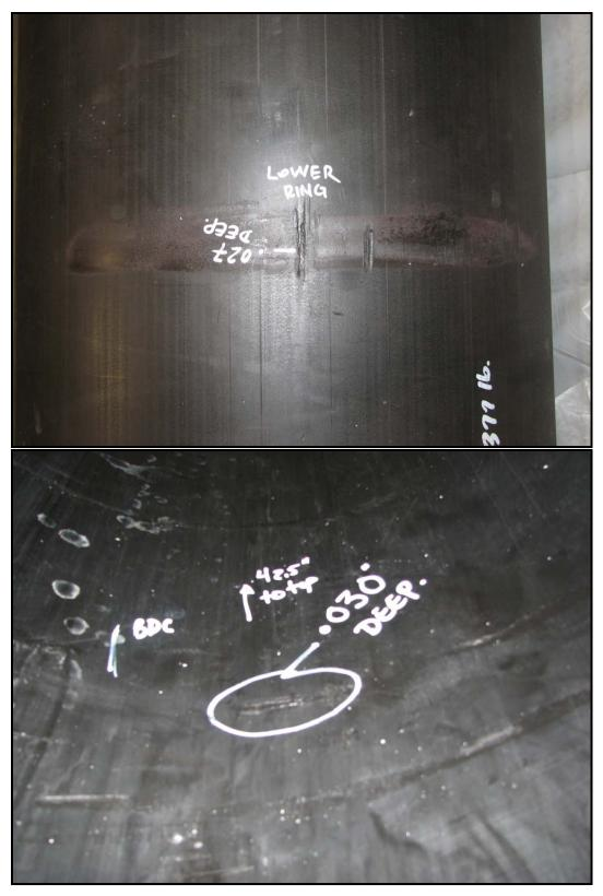
Figure 5.1-11 – Cold Drop Body Pipe Dents and Gouges
