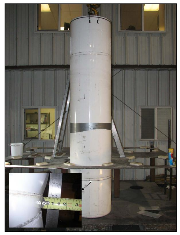
Figure 5.1-12 - Cold Drop Canister Metallic Component Deformations
