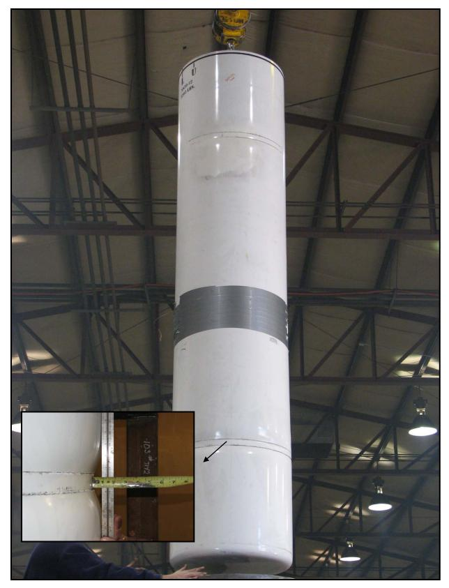
Figure 5.1-18 – Hot Drop Canister Metallic Component Deformations
