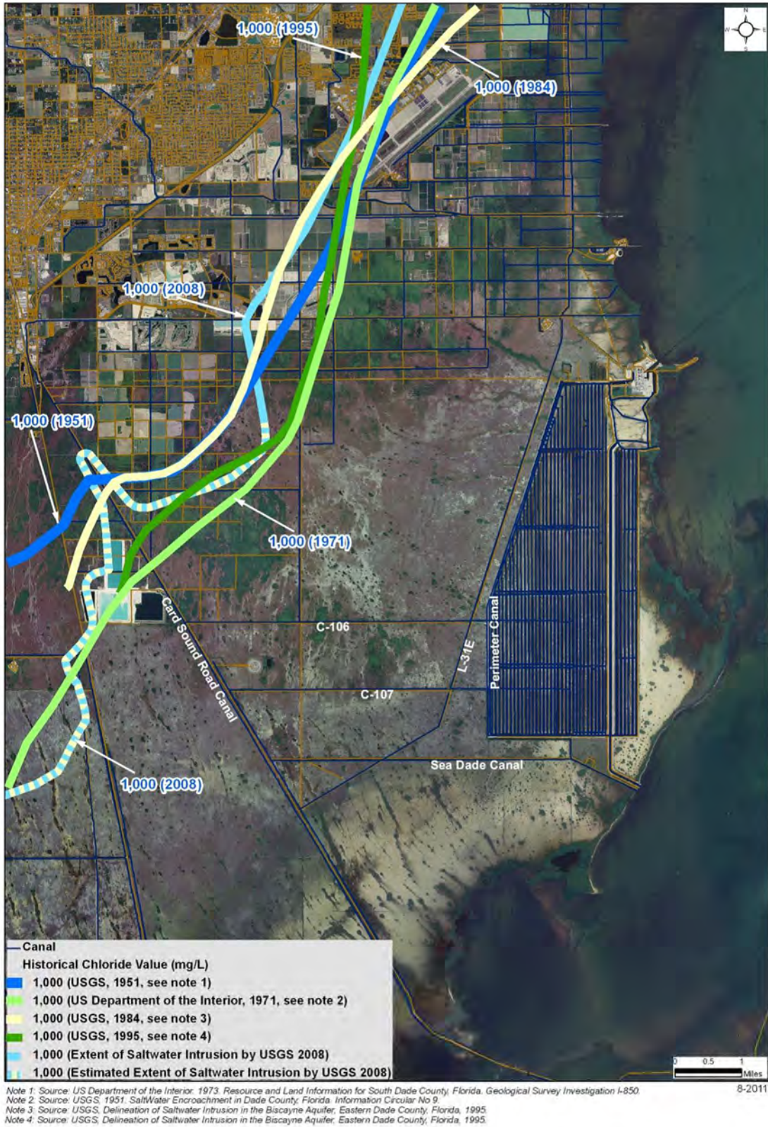
Figure 2-22. USGS Estimated Extent of Saltwater Intrusion from 1951 to 2008 (FPL 2012-TN3439)
