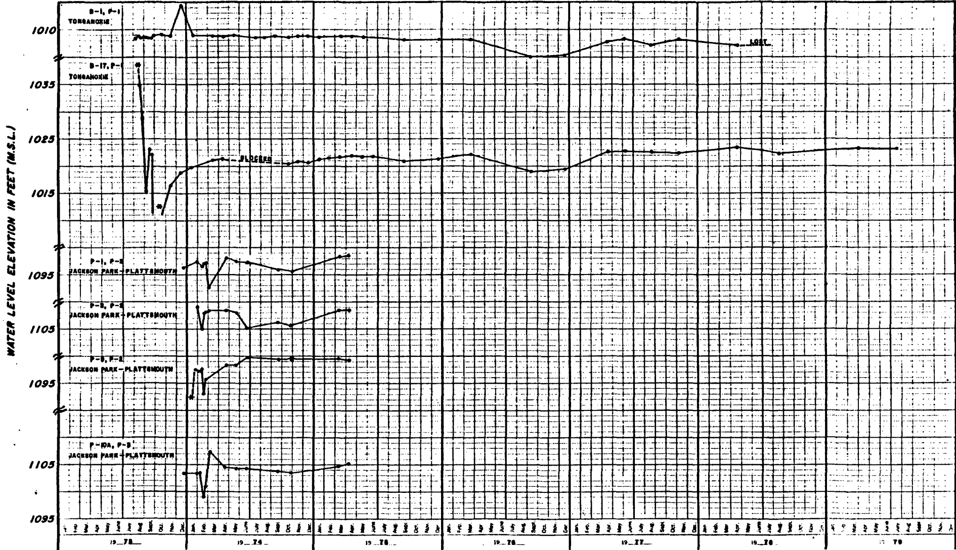
WOLF CREEK UPDATED SAFETY ANALYSIS REPORT Figure 2.4-56 (Sheet 10 of 18) Variations of Water Levels in Piezometers Rev. 0
