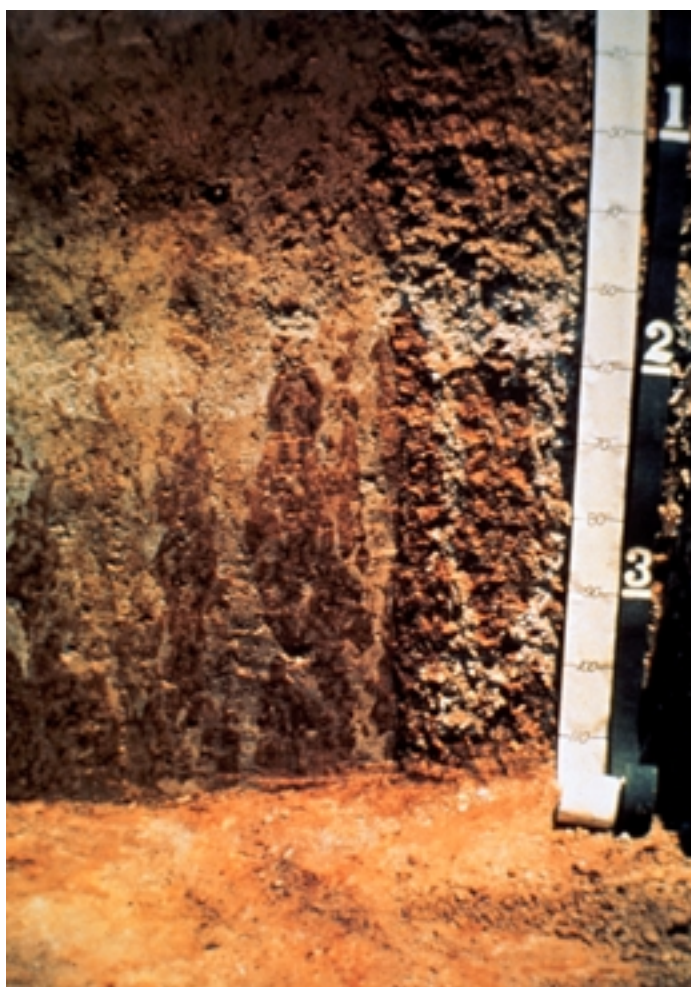
Photo 21.—A fragipan beginning at a depth of about 50 cm. Bleached seams are between the peds.
