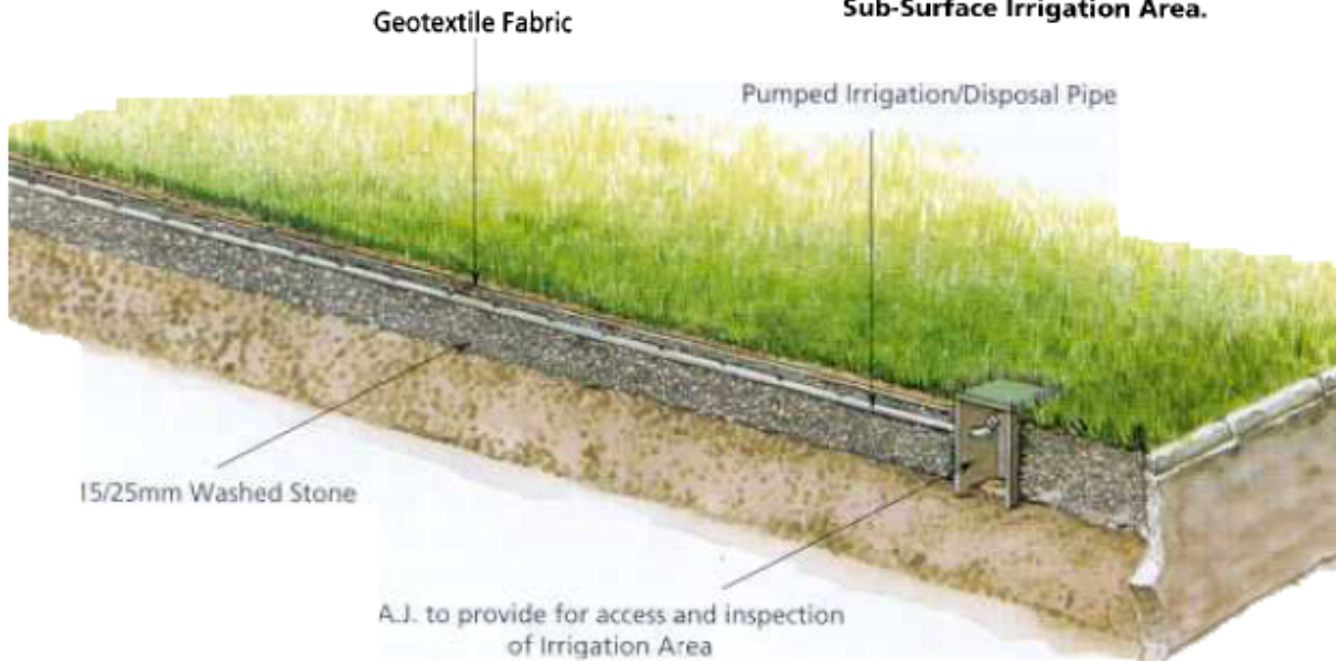
Fig. 3 Typical longitudinal section through Sub-Surface Irrigation Area.
