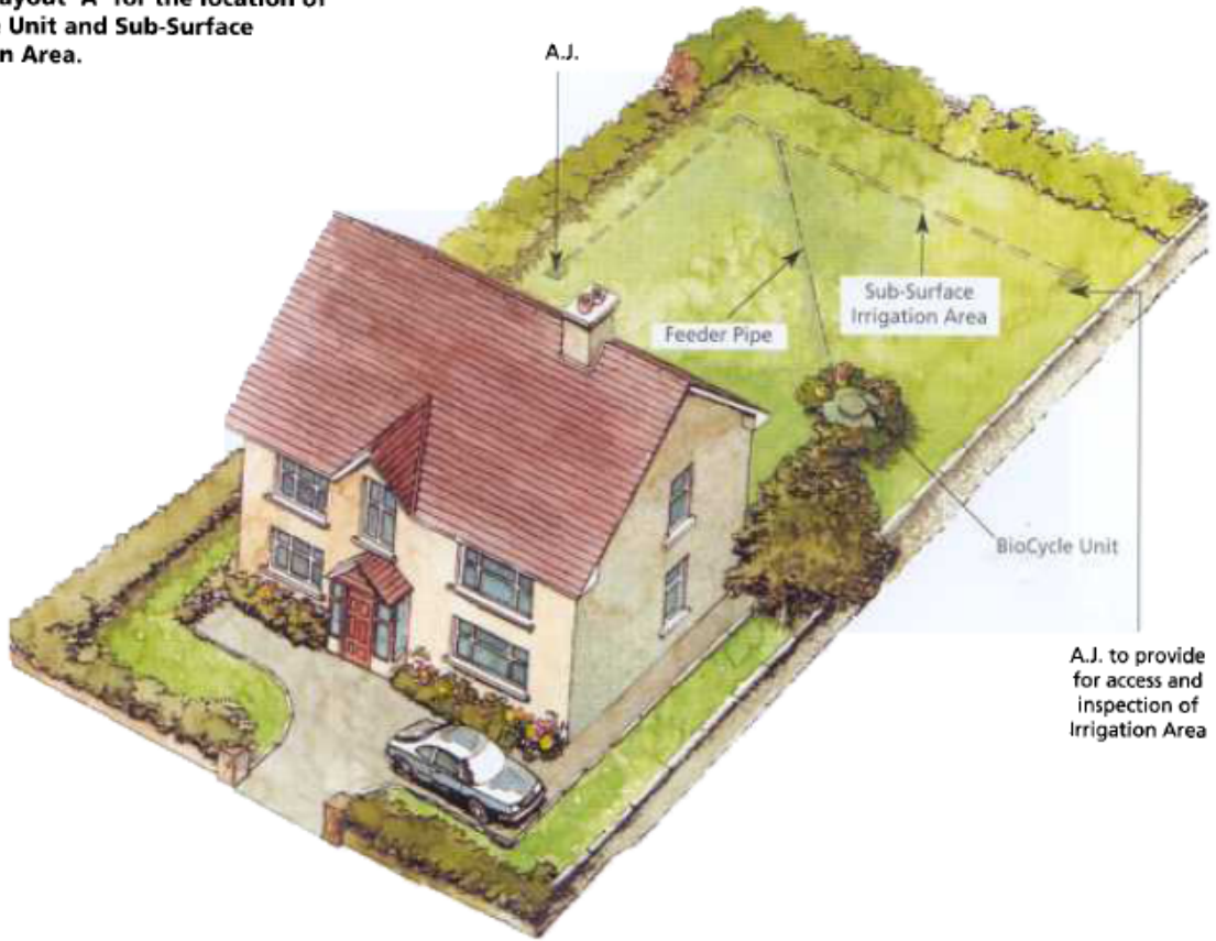
Fig. 7 Typical Layout 'B' for the location of BioCycle Unit and Sub-Surface Irrigation Area.
