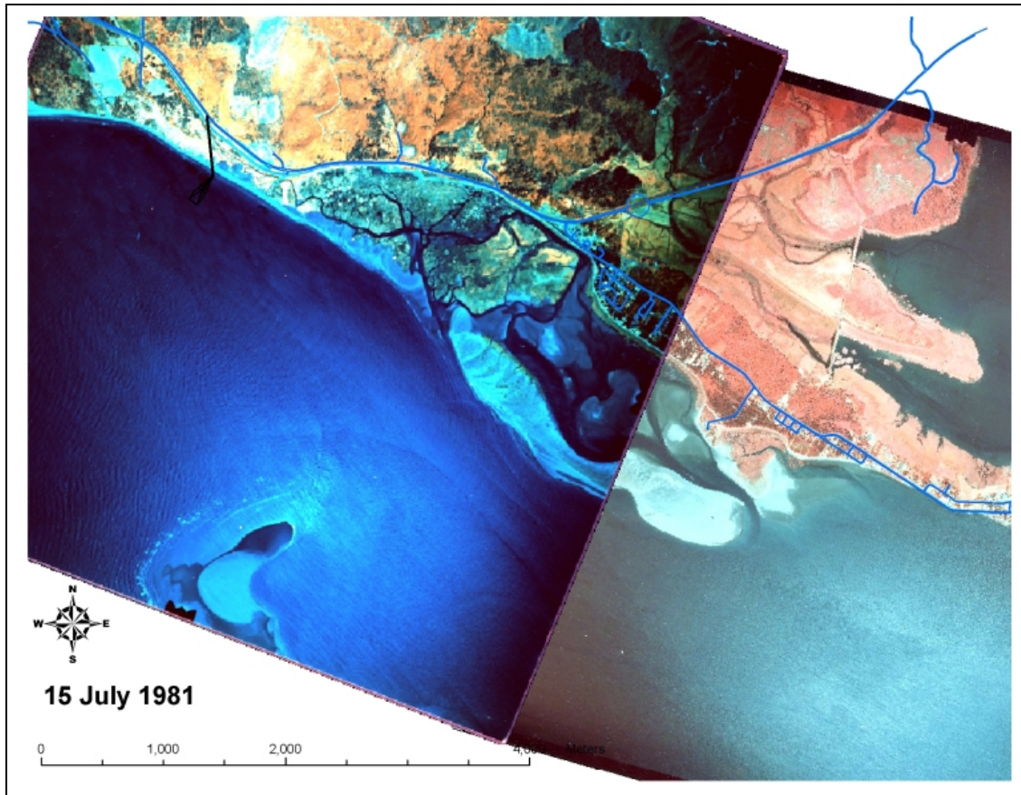
Figure 2.2. 12. 1981 aerial photograph. Original prints NWS. Note that Graveyard spit is thin and appears to have recently been overwashed.
