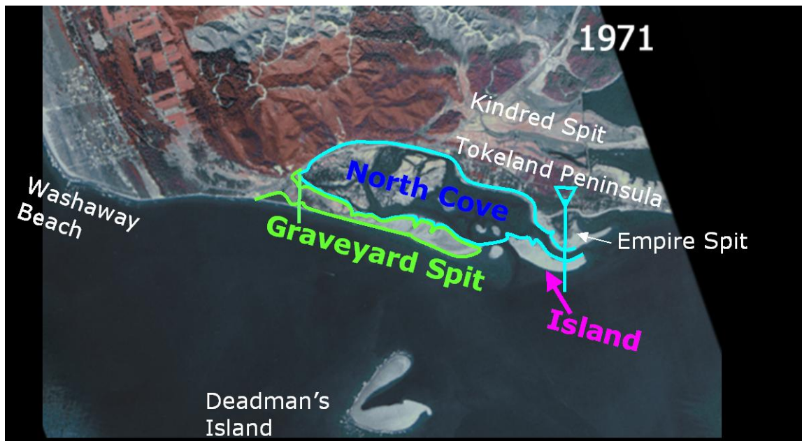
Figure 2.2. 43. Nomenclature and definitions of areas for which losses were quantified and for which causes and predictions are sought. A time series of annual changes in area were developed for each of the geomorphic features shown in bold (Spits, Islands, and North Cove).
